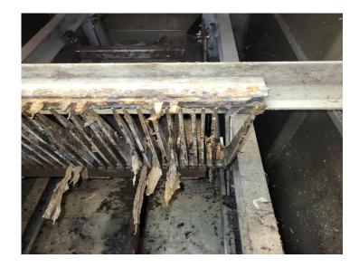
> The polypropylene rake and the leather must be changed
