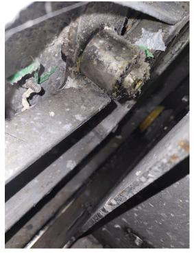
> The comb has teeth that are bent and should probably be replaced
